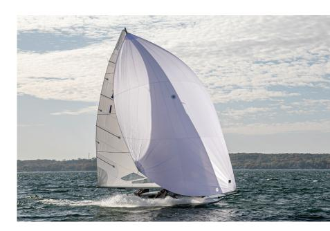
Crew weight should never exceed 675 lbs on an E Scow. The target weight for four people sailing in heavy wind is 630 lbs-650 lbs. Sailing heavier than that will dramatically increase loads on the boat and rigging and amplify mistakes made with tuning and mainsail handling.
